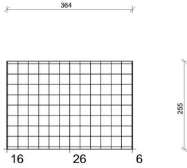
ARMATURA DI BASE SUP.=INF. SETTO 9 QUOTA m.64.95-68.17
